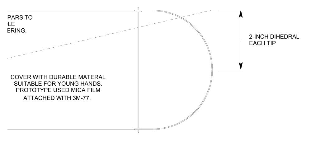
WITH D GLUE I DESIGNED AND BUILT THIS MODEL TO INTRODUCE MY THEN 3 1/2 YEAR-OLD NEPHEW TO THE JOYS OF FLYING MODELS. THE PROTOTYPE HAS BEEN FLOWN EXTENSIVELY AND, DESPITE HIS BEST EFFORTS, HAS REQUIRED ONLY A COUPLE OF REPAIRS IN THE LAST 7 YEARS. THE CARBON FIBER OUTLINES, DURABLE COVERING AND ROBUST FUSELAGE STICK HAVE PROVIDED A LASTING MODEL THAT CAN FLY FOR A MINUTE IN CALM AIR.
